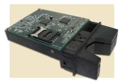
ID TECH's newest manual insert reader, the Compact Spectrum III, is one of the few readers in the industry that couples smart card and magnetic stripe reading capabilities into a compact solution. Available in RS232, RS-232 PC/SC, USB-CDC, and USB PC/SC interfaces, the Compact Spectrum III is a perfect fit for applications where space is at a premium, such as portable devices, handheld terminals or kiosks.
